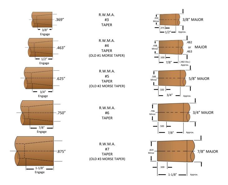
The above new R.W.M.A. tapers cover a broader range than the old Morse tapers. These new tapers are .600" taper per foot and replace the Morse tapers which vary from .5986 on the #1 M.T. to .6024 on the #3 M.T. The new R.W.M.A. #4, #5 and #7 tapers are inter-changeable with the old #1, #2 and #3 Morse tapers. You will note there are 2 new sizes, the #3 & #6 R.W.M.A. tapers.
